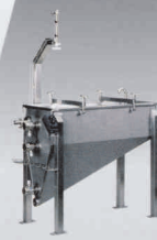
Container emptying station for remnant-free emptying of transporting containers, such as buckets with paste or extracts
