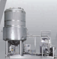
Processing system for cosmetic premixes, batch size 6.000 l
