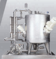
Production of emulsions, batch size 1.000 l
