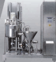
Universal pilot plant system for the production of emulsions and suspensions, batch size 100 l
